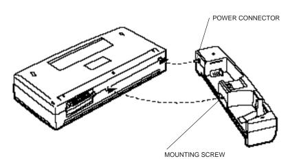
5. Fasten the battery case to the printer by turning the thumbwheel to the right (toward the  $\frac{1}{12}$  mark).
